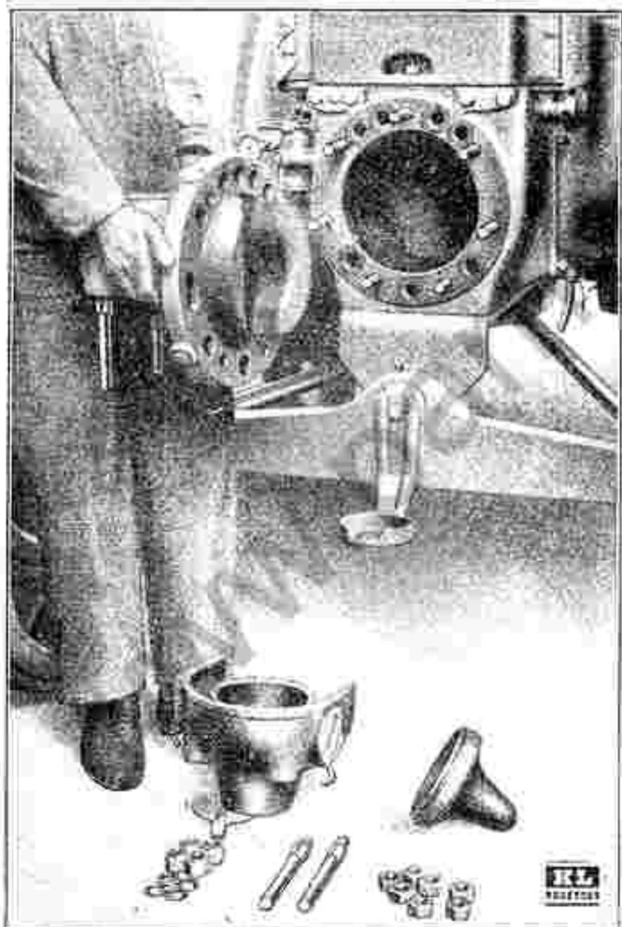
Fig. 49. Cylinder head removed.
