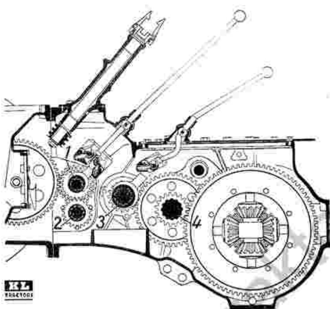
Fig. 67. Sectional view of transmission.
