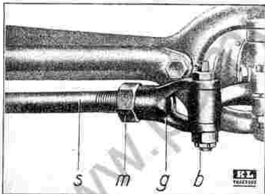
Fig. 78. Track rod adjustment.
