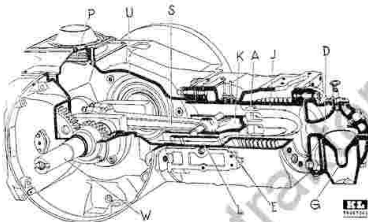
Fig. 2. Sectional view of the engine.
